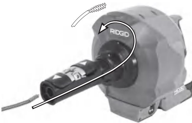
Figure 21 – Loading Cable Without Changing Inner Drum
