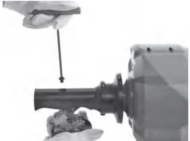
Figure 16A – Removing AUTOFEED Mechanism
