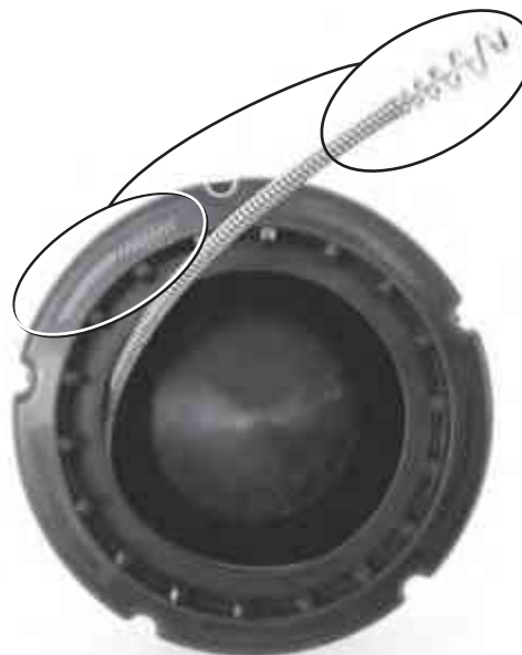
Figure 20 – When Loading Cable Into An Inner Drum, Coil The Cable CLOCKWISE
